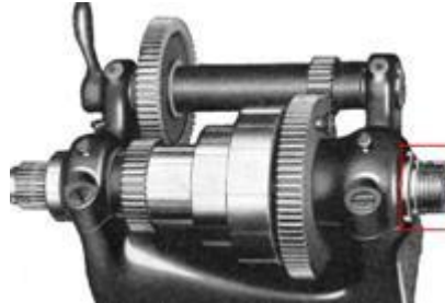
Head Stock With Threaded Spindle Nose (Head Stock and back gear shown uncovered) Face Plate and Chuck thread onto the spindle nose outlined in red. Note back gear lever at upper left.
