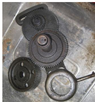
Banjo Bracket and Gear Assembly removed
