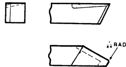
Fig. 47. Detail of Roughing Tool Bit
