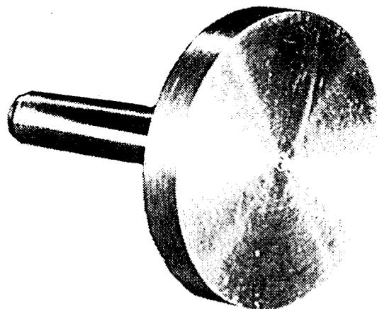
Fig. 133. Drill Pad for Use in Tailstock
