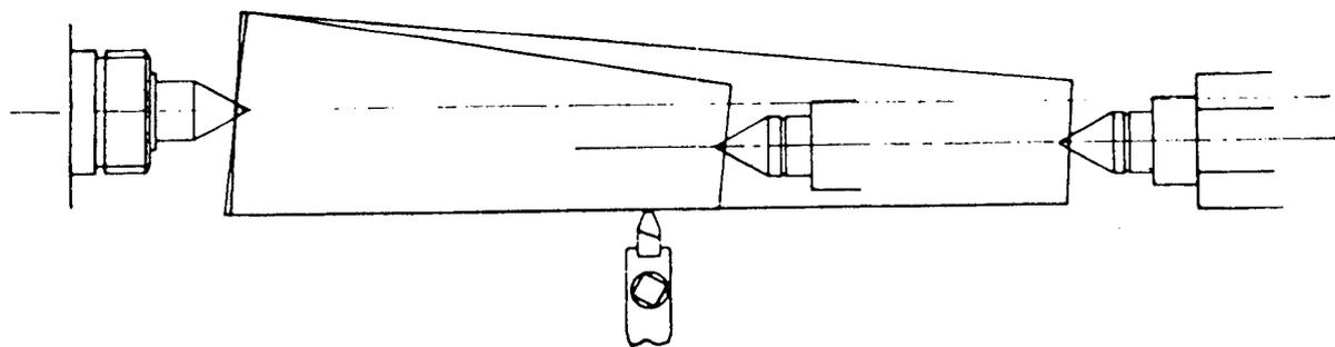
Fig. 110. Diag. to show Different Taper on different lengths with same Tailstock Offset
