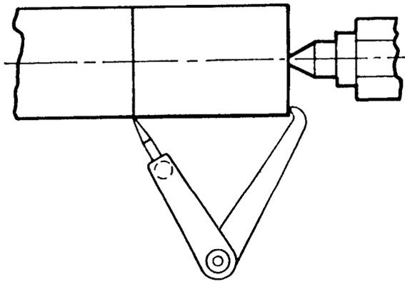
Fig. 101. Locating a Shoulder with Hermaphrodite Caliper
