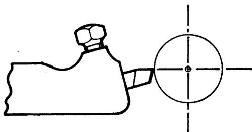
Fig. 36. Tool Cutting Edge on Centre
