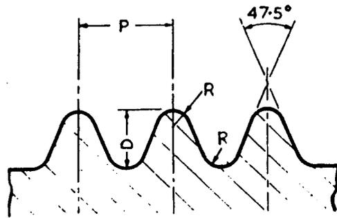
Fig. 178. British Association (B.A.) Screw Thread Form
