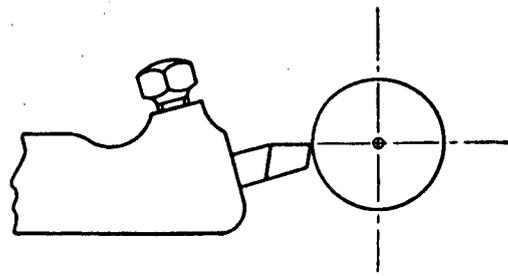
Fig. 62. Brass Turning Tool
