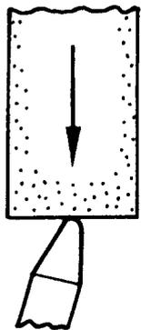
Fig. 43. Rounding Tool Bit
