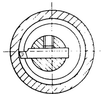
Fig. 160. Cutting Edge of Tool Bit Set on Centre for Internal Threading
