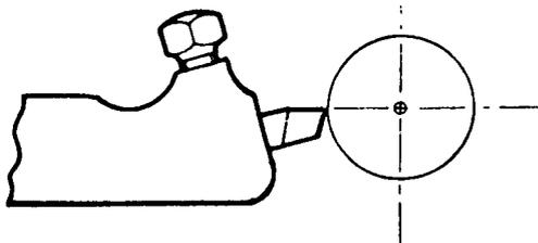
Fig. 60. Thread Cutting Tool
