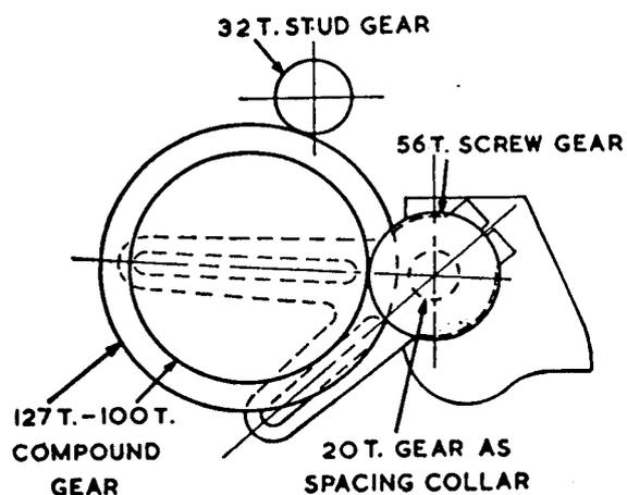
Fig. 185. Diagram showing standard English Change Gear Lathe Set Up for Cutting 4 mm Pitch Thread
