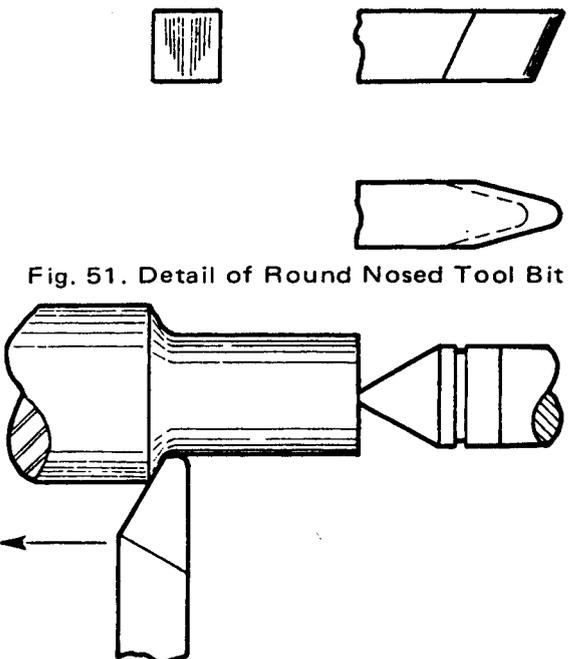
Fig. 51. Detail of Round Nosed Tool Bit
