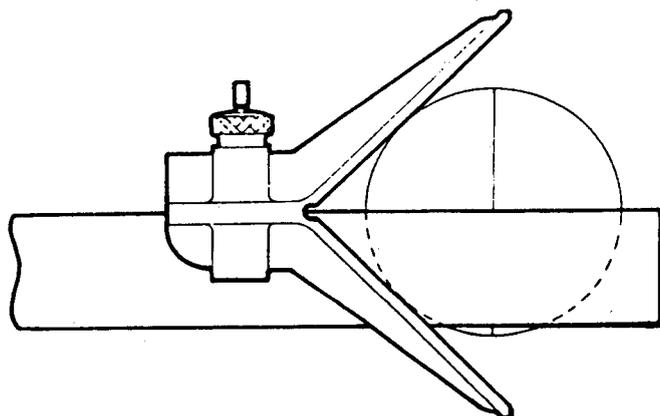
Fig. 83. Combination Square Centre Head to Locate Centres
