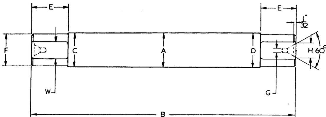
Fig. 224. Taper Mandrel for Machining Work between Centres
