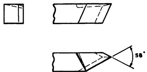
Fig. 59. Detail of Left-Hand Facing Tool Bit
