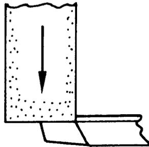
Fig. 44. Grinding Side and Back Rake of Tool Bit
