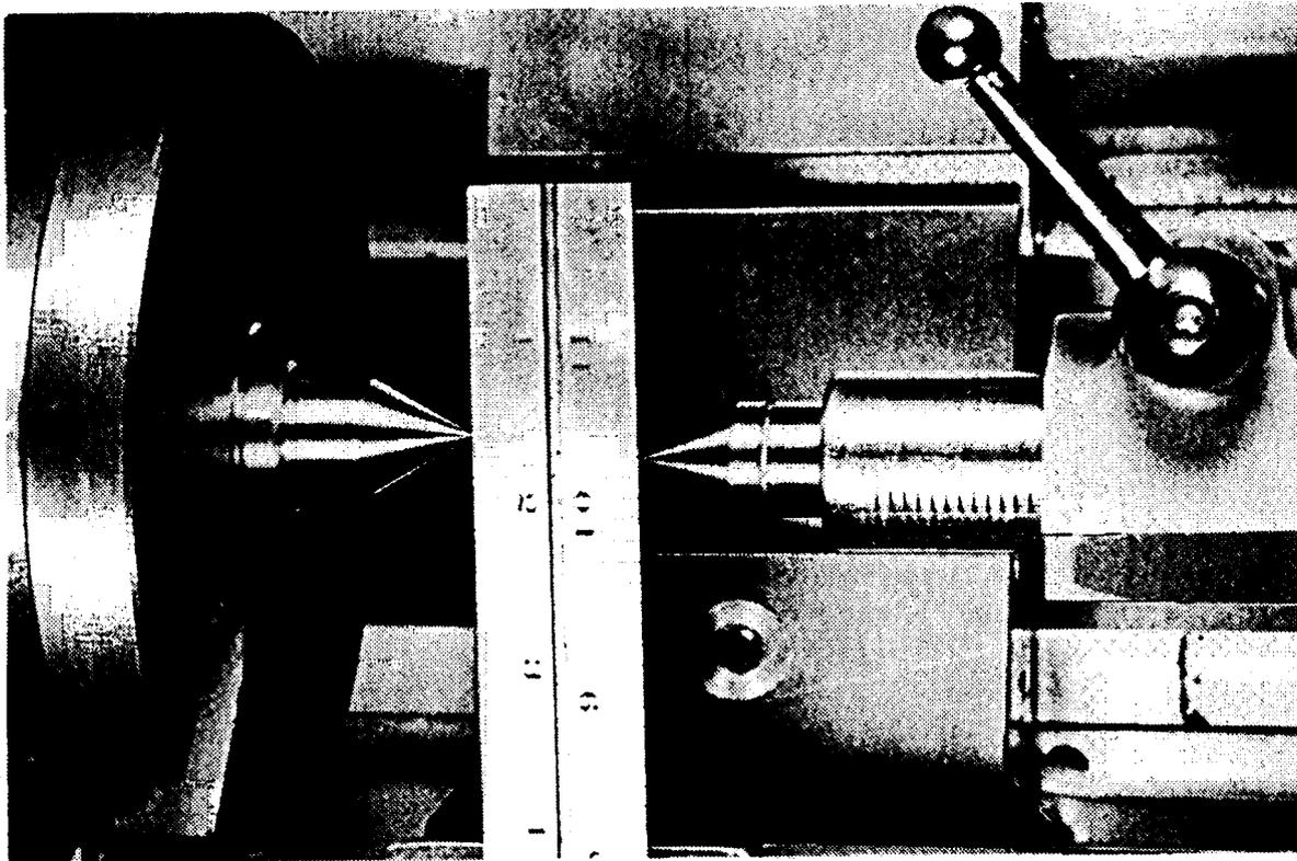
Fig. 112. Measuring the Amount of Offset
