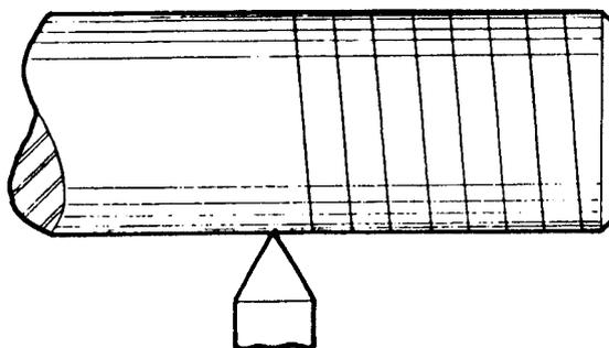
Fig. 169. Taking a Trial Cut
