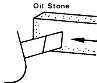
Fig. 45. Honing Cutting Edge of Tool Bit
