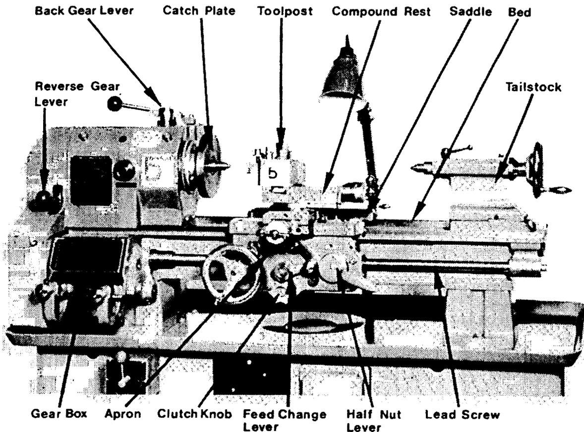
Fig. 11. The Main Parts of a Lathe
