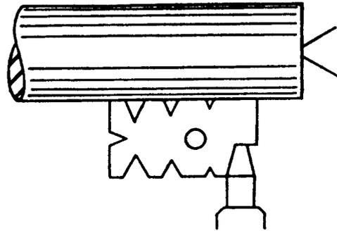
Fig. 182. Setting Tool for Cutting Acme Thread
