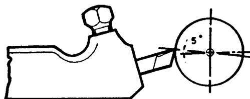
Fig. 35. Tool Cutting Edge above Centre
