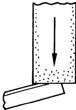
Fig. 40. Grinding Left Side of Tool Bit
