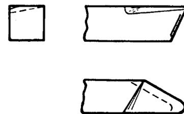
Fig. 49. Detail of Finishing Tool Bit
