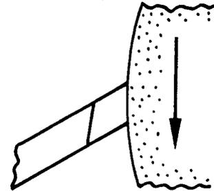
Fig. 42. Grinding Front of Tool Bit
