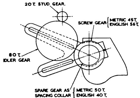
Fig. 153. Diagram of Standard Set Up on Model A Lathes
