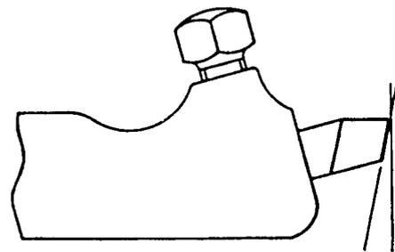
Fig. 157. Side View of Tool Bit showing Front Clearance
