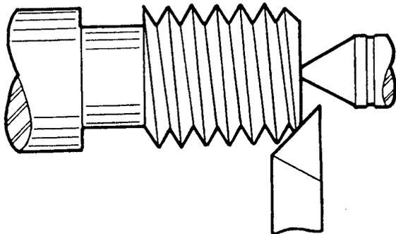
Fig. 172. 45° Chamfer at End of Thread
