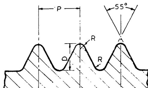
Fig. 145. B.S. Whitworth Thread Form
