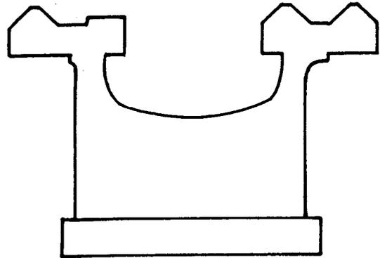
Fig. 8. Lathe Bed Formation
