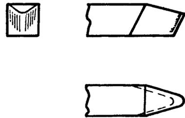
Fig. 63. Detail of Brass Turning Tool Bit
