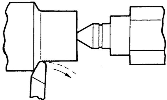
Fig. 98. Position of a Tool Bit for Turning
