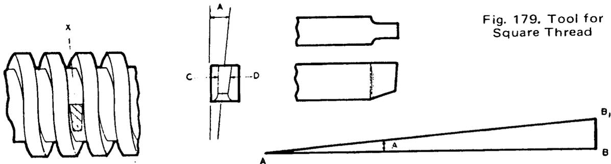
Fig. 179. Tool for Square Thread
