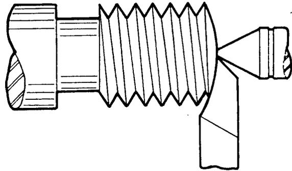
Fig. 173. Finishing End with Form Tool
