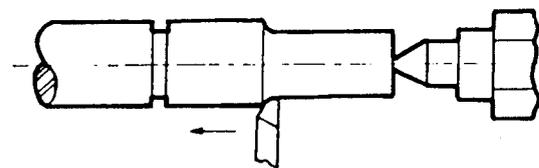
Fig. 104. Locating Shoulder with Parting-off Tool
