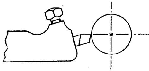
Fig. 158. Tool Bit Set on Centre for Cutting Screw Threads
