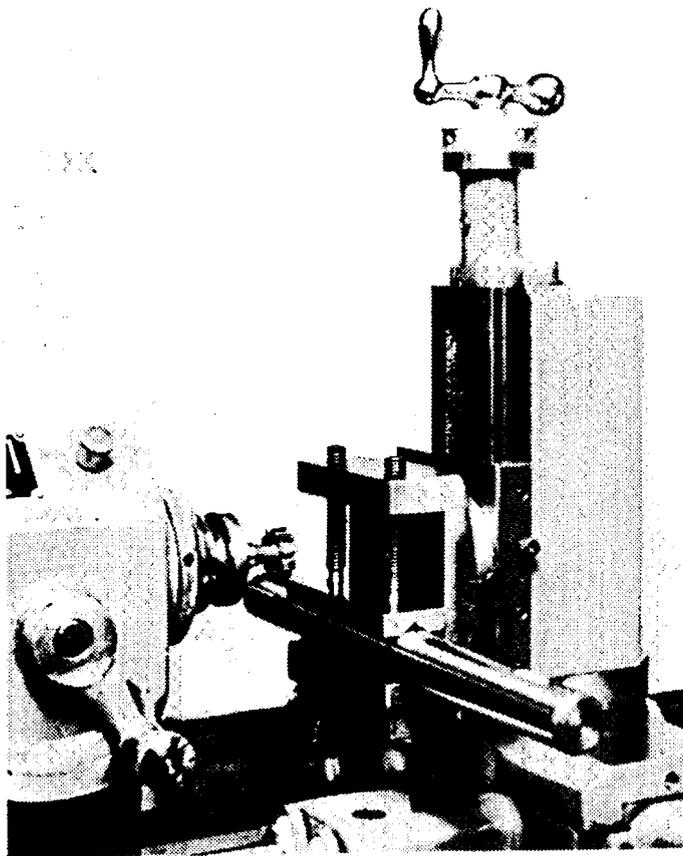
Fig. 210. Milling Attachment in Use
