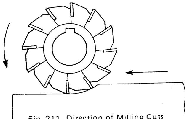
Fig. 211. Direction of Milling Cuts
