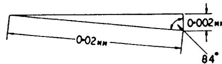
Fig. 78. Compound Rest Set for Fine Cross-Feed
