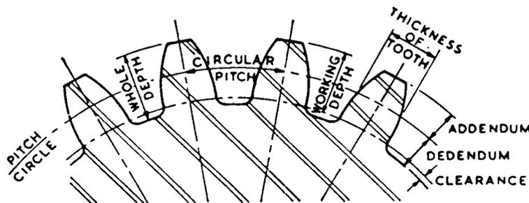
Fig. 226. Gear Tooth Names
