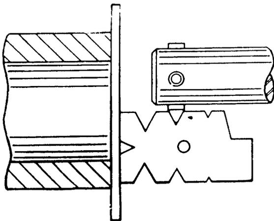
Fig. 161. Tool Bit Set Square for Internal Threading
