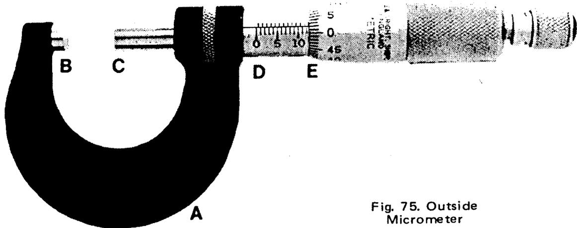
Fig. 75. Outside Micrometer
