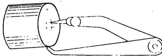
Fig. 86. Centring a Shaft with Hermaphrodite Caliper
