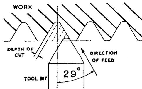
Fig. 166. Cutting Action of Tool Bit when Compound Rest is Set at Angle
