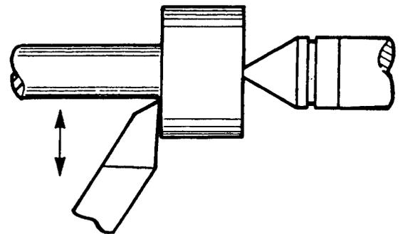
Fig. 58. Left-Hand Facing Tool Bit
