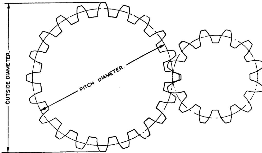
Fig. 225. Spur Gearing (Involute)
