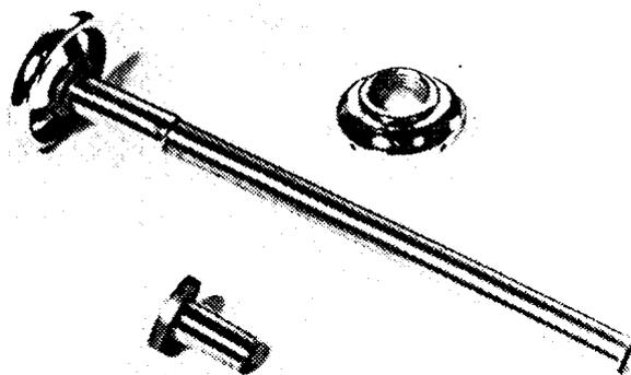
Fig. 127. Draw-Bar, Collet Adaptor and Nose Cap
