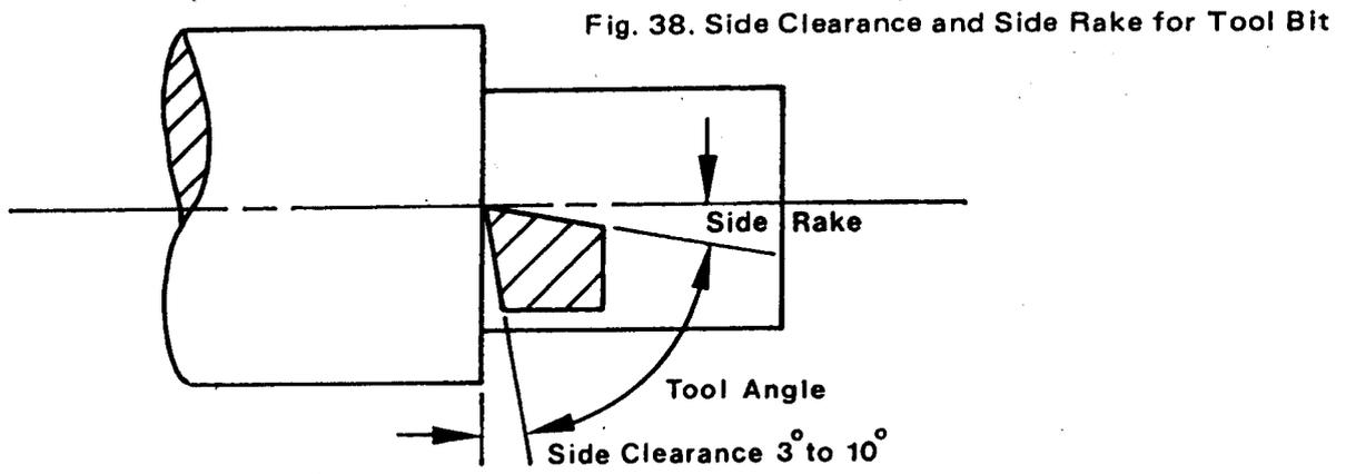
Fig. 38. Side Clearance and Side Rake for Tool Bit
