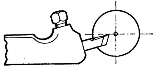
Fig. 96. Tool Bit Position for Facing End of Shaft
