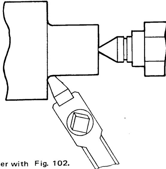
Machining a Fillet Corner with Fig. 102. Round-Nosed Tool
