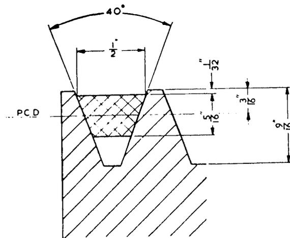
Fig. 228. Vee Pulley Dimensions for "A" Section V-Belts
