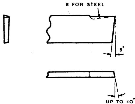
Fig. 65. Detail of Parting-off Blade
