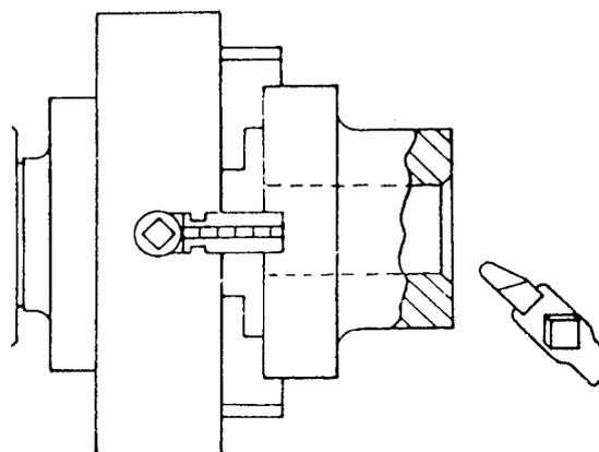
Fig. 137. Chamfering Cored Hole to start drill true
