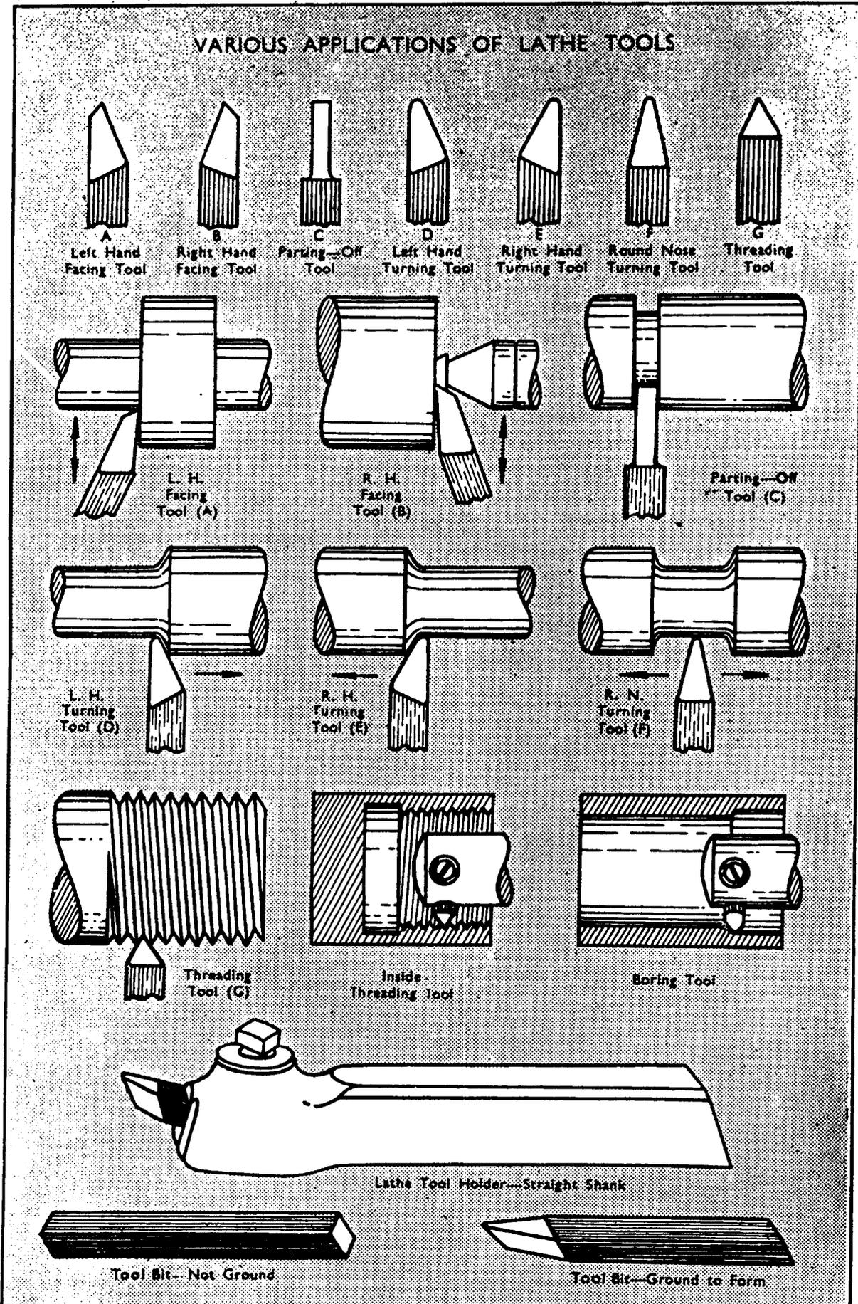
Fig. 68. Tool Bit Shapes and Applications
