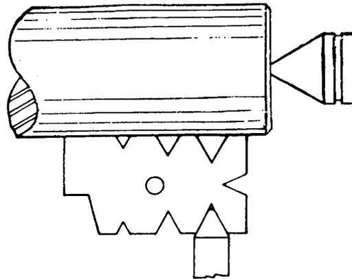
Fig. 159. Tool Bit Set Square for External Screw Thread
