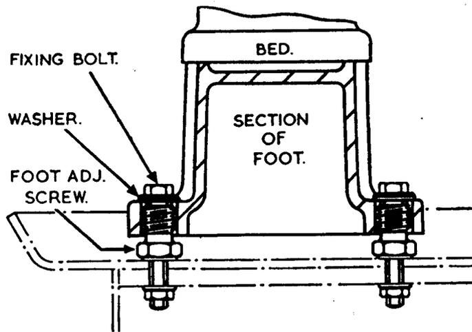
Fig. 20. Lathe Foot with Levelling Screws
