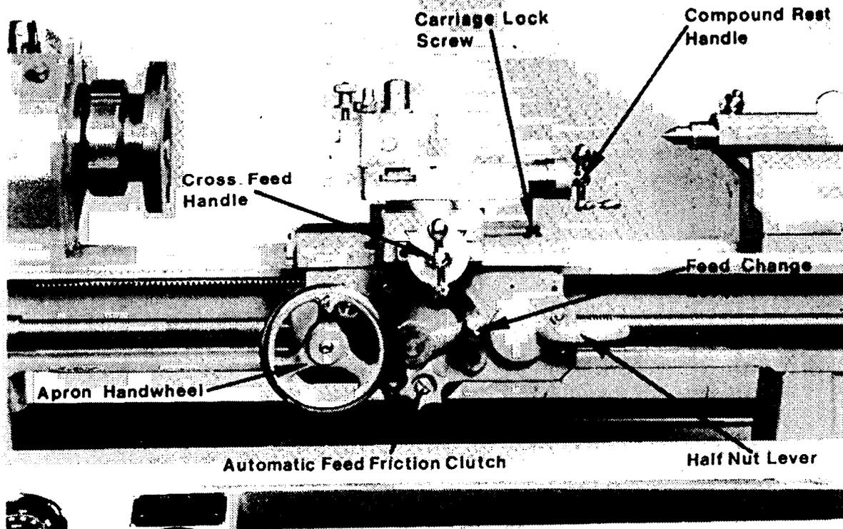
Fig. 14. Operating Parts of Lathe Carriage and Apron
