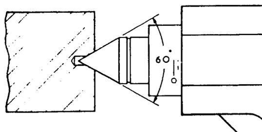
Fig. 91. Correctly drilled Centre Hole
