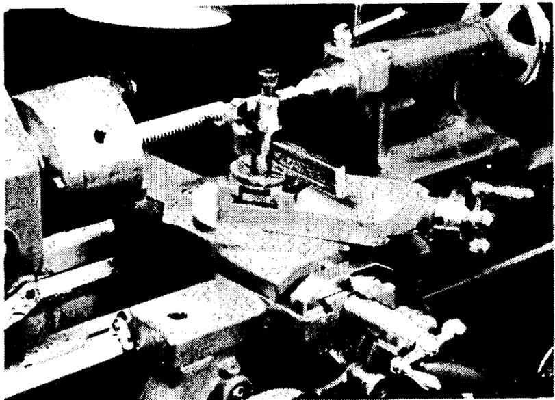
Fig. 167B. Thread Cutting Stop in Use
