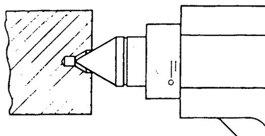
Fig. 92. Centre Hole Drilled too Deep
