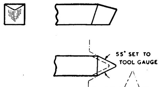
Fig. 61. Detail of Thread Cutting Tool Bit
