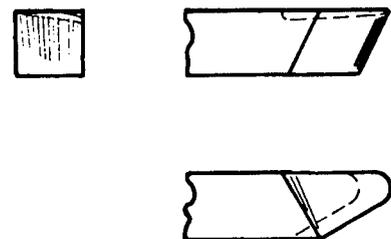
Fig. 55. Detail of Left-Hand Turning Tool Bit
