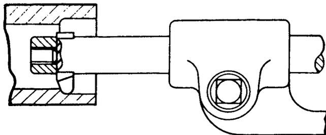
Fig. 67. Boring Tool Bit and Boring Bar
