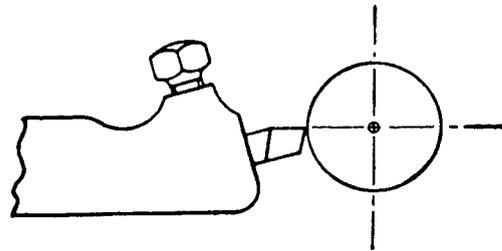
Fig. 105. Tool Bit on Centre for Taper Turning
