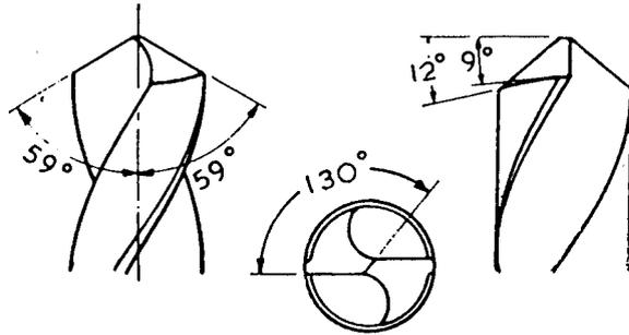
Fig. 138. Detail of Drill Point
