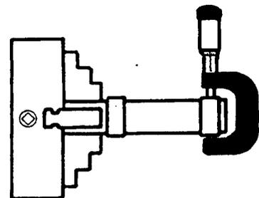
Fig. 21. Method of Checking Levelling of Lathe
