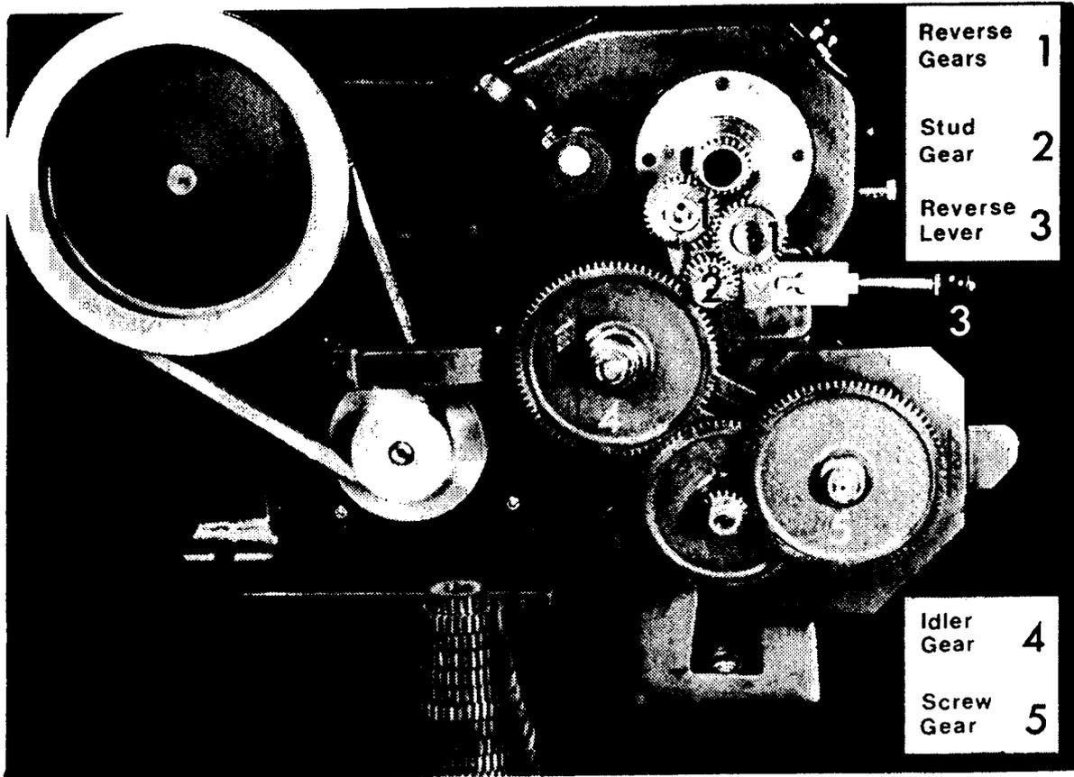
Fig. 149. Set up of Standard Change Gear Lathe for Cutting Screw Threads (Fig. 4 on gear chart)
