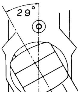
Fig. 165. Diagram showing Angle of Compound Rest for ISO Metric Threads
