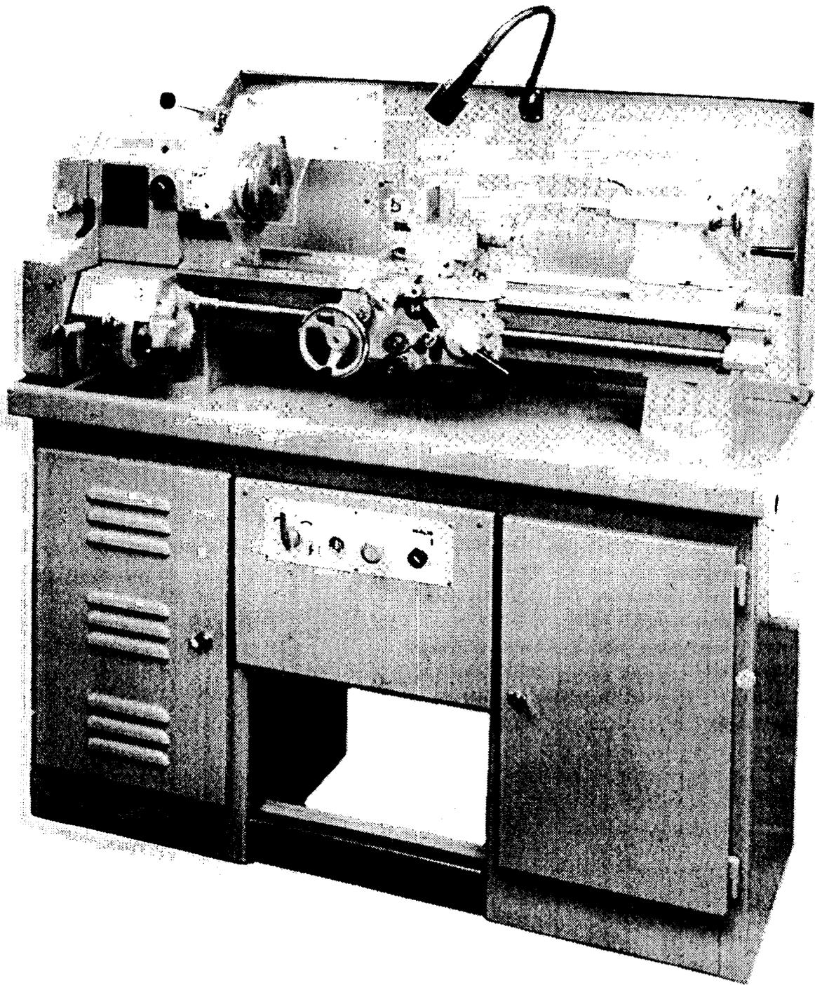
**Fig. 5. Underneath Drive Cabinet Mounted Lathe (Model AUD)**
