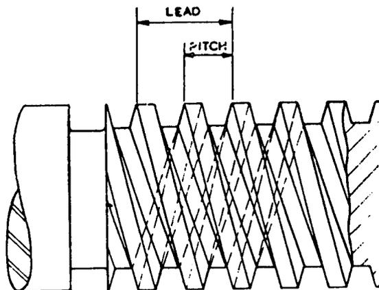
Fig. 189. A Double (or Two-Start) Thread
