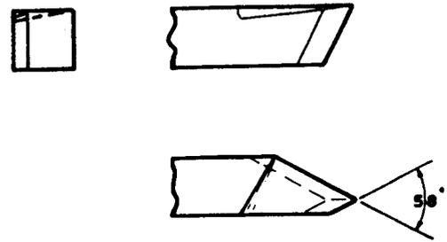
Fig. 57. Detail of Right-Hand Facing Tool Bit
