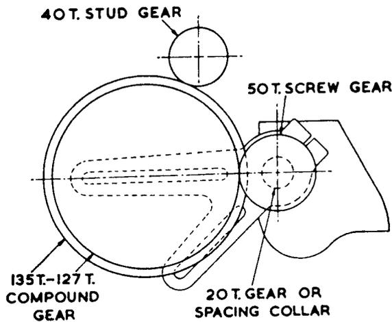
Fig. 186. Diagram showing standard Metric Change Gear Lathe Set Up for Cutting 10 T.P.I.
