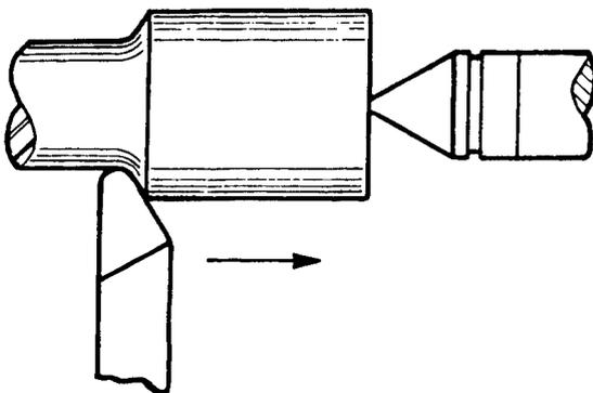
Fig. 53. Detail of Right-Hand Turning Tool Bit
