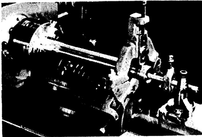
Fig. 205. Work Held in Chuck Supported at Free End by Fixed Steady
