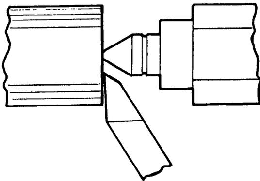
Fig. 97. Facing the End of a Shaft
